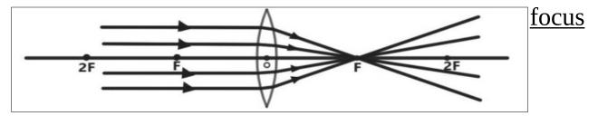
Light rays near and parallel to the optic axis incident on a convex lens, after refraction converge at a point on the optic axis
