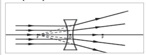
Light rays, near and parallel to the optic axis incident on a concave lens, after refraction appear to diverge from a point on the optic axis on the same side of the lens. This point is the principal focus of a concave lens (F).
