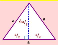
Let the length of one side of an equilateral triangle be 'a' units. A vertical draw from vertex to base bisects the triangle divide into triangles with right angles.
