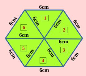
Here, the area of regular hexagon =  $6 \times$  Area of an equilateral triangle side of an equilateral triangle = 6 cm
