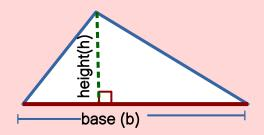
If the height is h and the base is b, then the area of the triangle =  $\frac{1}{2}$  ×base ×height
