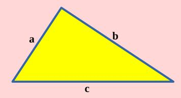
Area of the triangle =  $\sqrt{s(s-a)(s-b)(s-c)}$ Here 's' is half of the perimeter,  $s = \frac{a+b+c}{2}$
